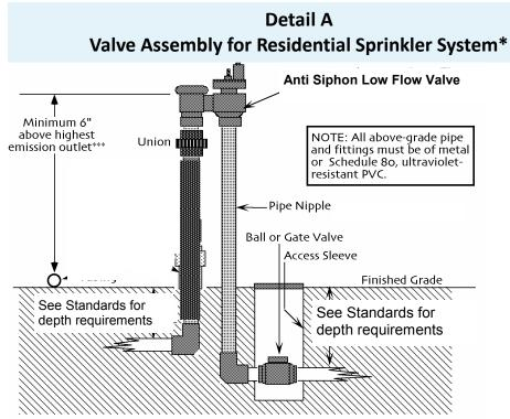
\* The minimum flow rate of the valve must be equal to or less than the flow rate of the zone. \*\* Optional if Master Device installed at Point of Connection \*\*\* For container zones this dimension must be at least six inches above the rim of the highest container.
