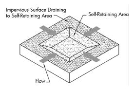
Figure 4-2. Ratio of impervious area draining to a self-retaining area shall be no more than 2:1.
