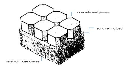
Typical configuration for a pervious pavement. The base course is a minimum 3" depth for runoff retention. A deeper base course is typically required for pavement stability.
