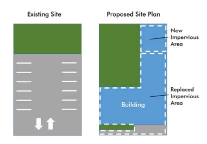
Figure 3-1. Illustration of Replaced Impervious Area.
