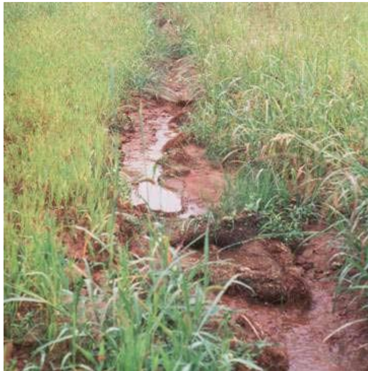
WITHOUT EROSION CONTROL MATTING CHANNEL FAILURE
