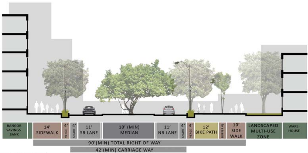
SECTION D-D' Through Franklin Street Near Fore St. Looking North
